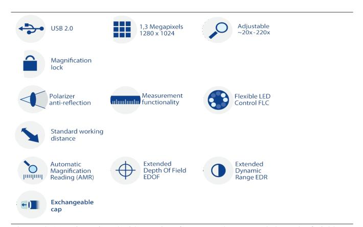
The WF4915ZT is equipped with premium features such as Extended Depth of Field (EDOF), Extended Dynamic Range (EDR), Flexible LED Control (FLC), integrated polarizer, extensive measurement functionality and Automatic Magnification Reading
